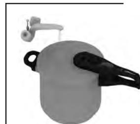
**Automatic Release Method:** remove the pressure cooker from the heat source, place the working valve or pressure regulating valve in the steam release position so that the steam is completely released and the lid can be safely removed.
